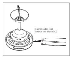
**C.** Tighten screws provided in kit. Refit the top motor housing to the fan body by reversing step1.
