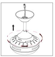
**B.** Insert the blade into the rectangular slot on the side of the motor body.
