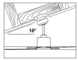
This fan hanging system supports a maximum 18° angled ceiling installation.
